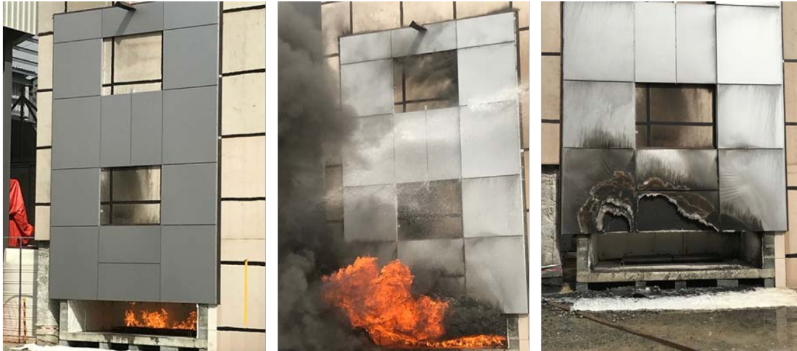
Figure 5 - Photos depicting the T2 fire scenario shortly after ignition (left), fully developed approximately 5-7 minutes after ignition (center), and subsequent damage (right) for the horizontal attack test.
