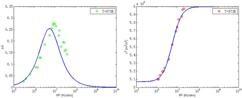
Fig. 2. (a) Acoustic absorption in hydrogen. (b) Sound speed in hydrogen.  $T=873\text{ K}$ , blue curve represents the spectrums predicted by the model of this work at the same temperature, green and red circles represent the experimental data from the literature [9].
