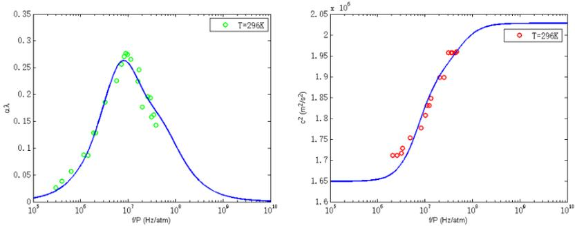
Fig.1. (a) Acoustic absorption in hydrogen. (b) Sound speed in hydrogen.  $T=296\text{ K}$ , blue curve represents the spectrums predicted by the model of this work at the same temperature, green and red circles represent the experimental data from the literature [9].
