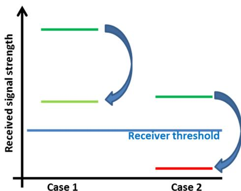
Fig. 5. Principle of test for immunity to site attenuation.
