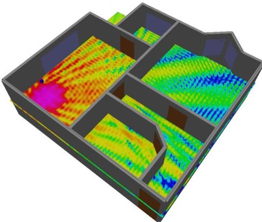
Fig. 1. Example of software prediction of coverage (RSS).
