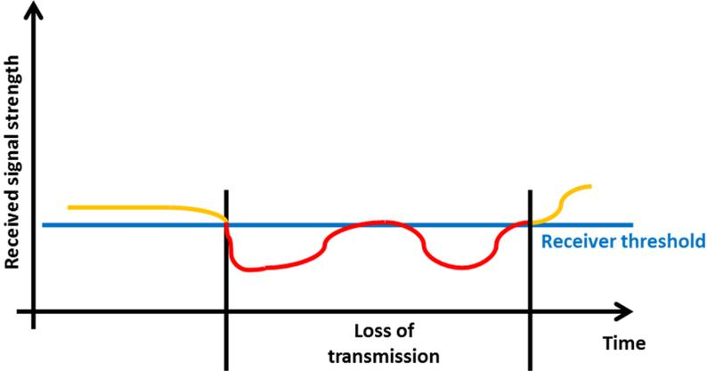
Fig. 4. Variation of the received signal strength and loss of transmission during some period.
