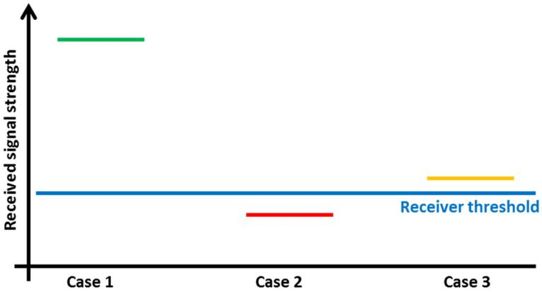
Fig. 3. Margin between received signal strength and receiver threshold: 3 cases.
