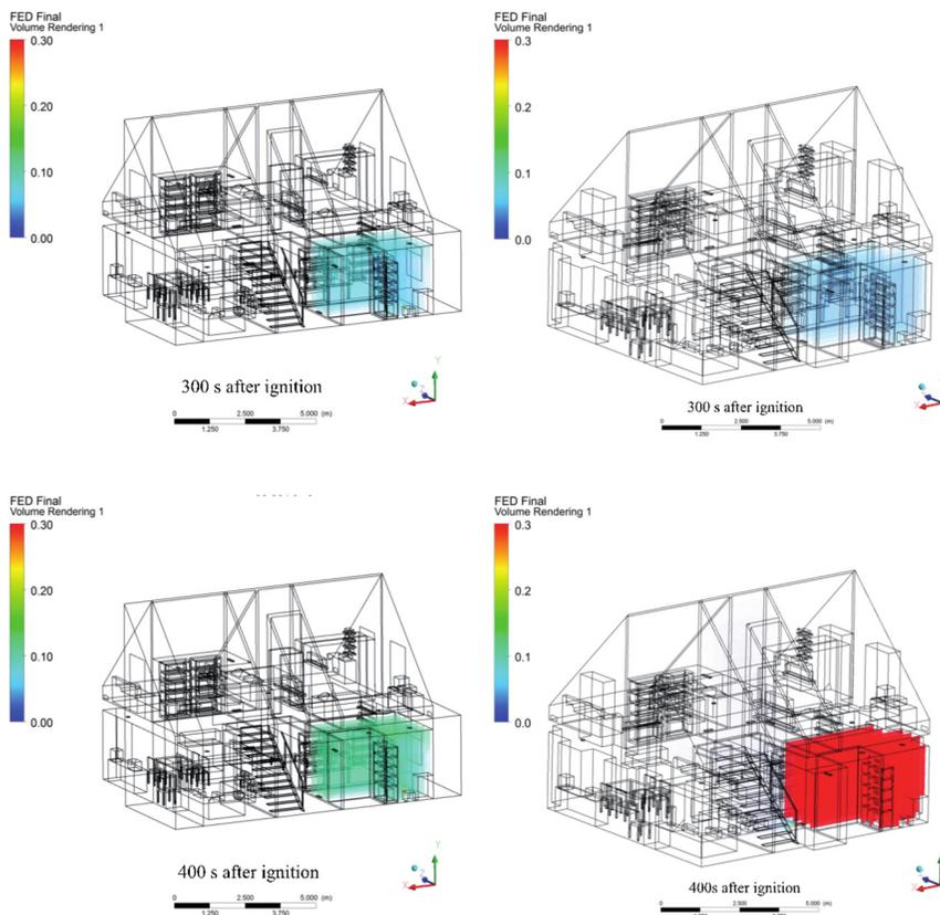
Fig. 6 Iso-volume with a FED value less or equal to 0.3 for a window ventilated fire on the left side and for a dwelling with mechanical ventilation system on the right side.
