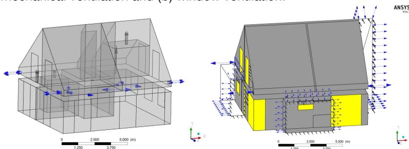
Fig. 2. Geometry of the house and boundary conditions (a) mechanical ventilation system; (b) window ventilation.
