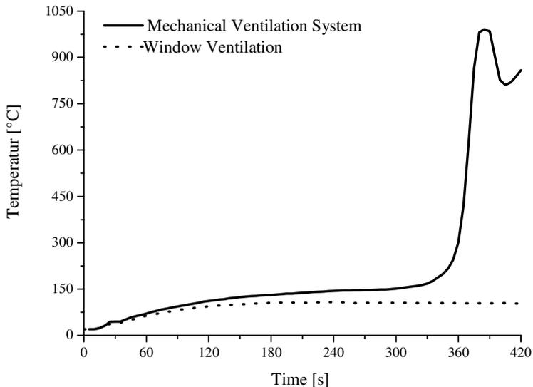
Fig. 3 Temperature vs. time in the utility room, 1.8 m above floor surface.
