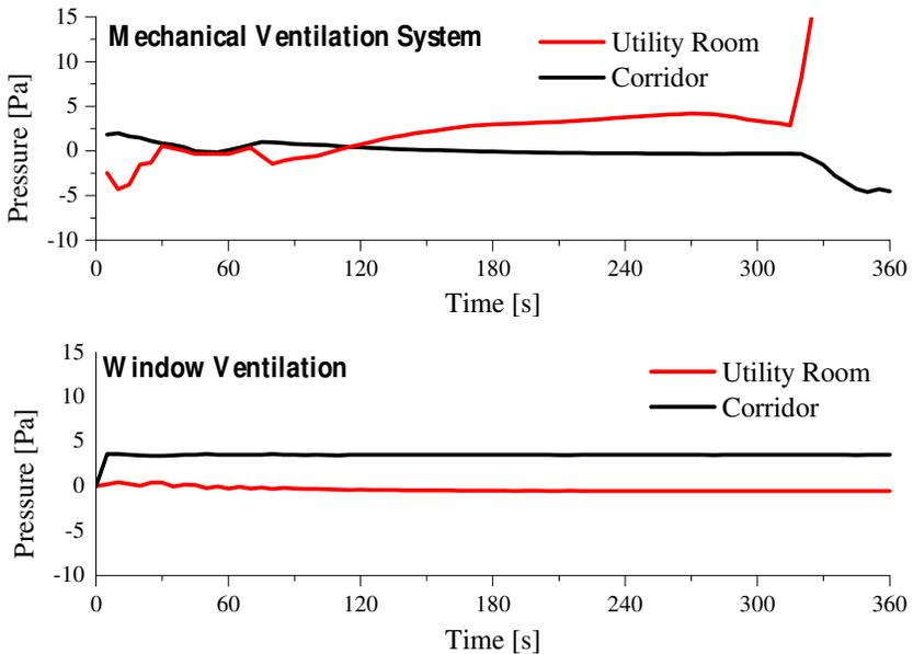
Fig. 5 Pressure vs. time curves for different ventilation conditions.
