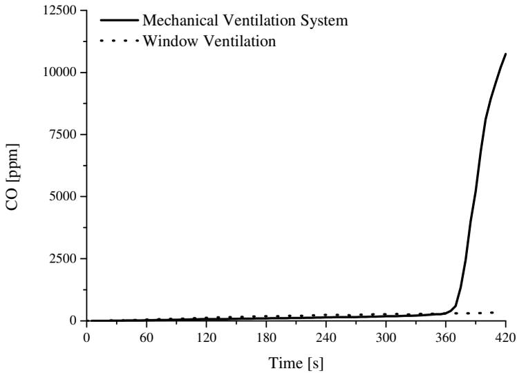
Fig. 4 CO Concentration vs. time in the utility room, 1.8m above floor surface
