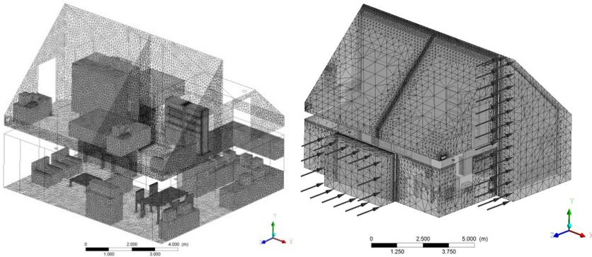
Fig. 1. Computational domain with tetrahedral mesh (a) mechanical ventilation system; (b) window ventilation.
