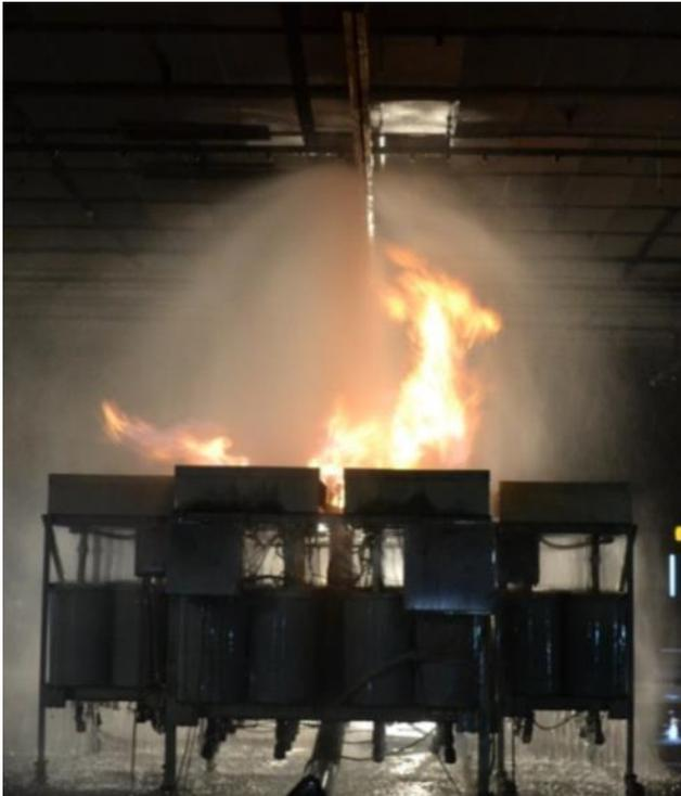
Figure 3. ADD Testing Apparatus With Obstruction.
