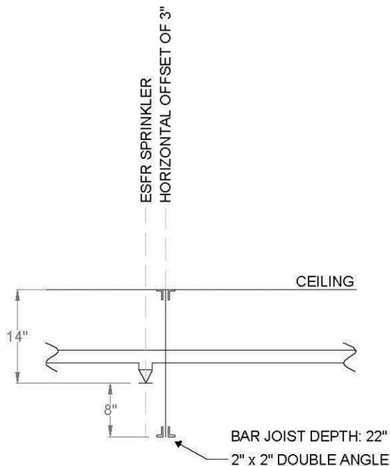
Figure 2. Typical Sprinkler Obstruction Arrangement.
