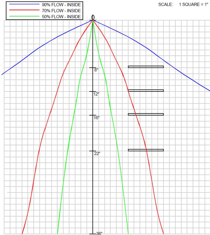
Figure 4 . ESFR K17 Sprinkler Spray Pattern with 6-Inch Wide Flat Obstruction Horizontally Offset 6 Inches
