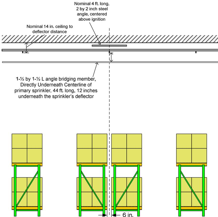
Figure 6. Typical Full Scale test Arrangement, Elevation View Near Ceiling
