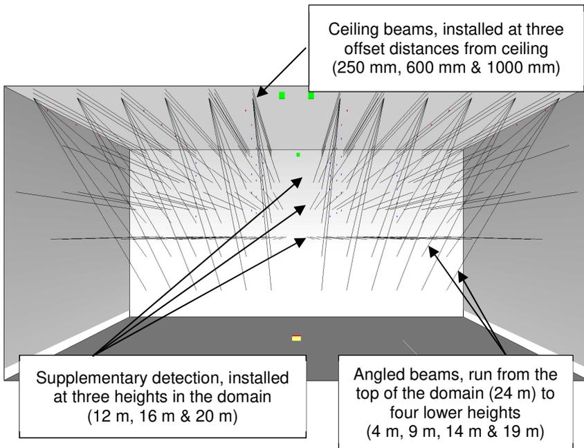
Fig. 1. General arrangement of beam detectors installed in the domain.
