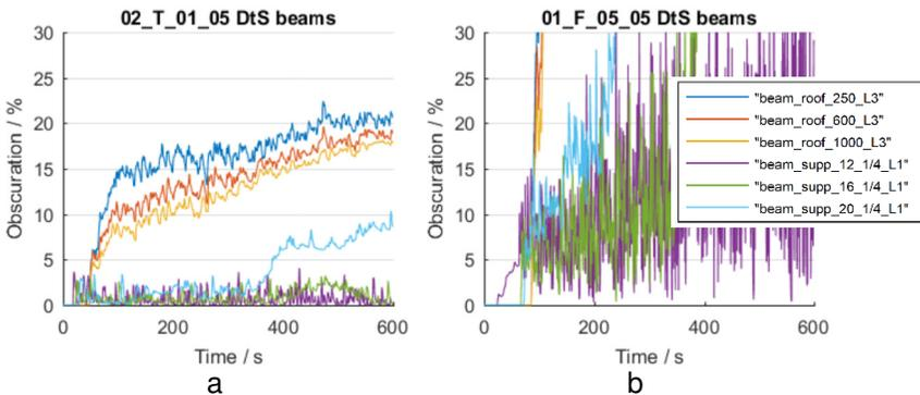
Fig. 4. Response of “code-compliant” beams to a 5 kW fire (with no  $\Delta T$ ) and to a sofa fire (with  $\Delta T=0.5$  °C/m).
