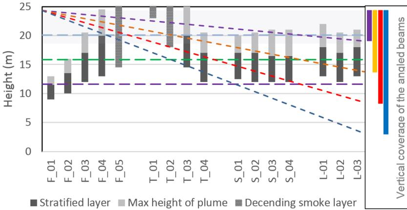
Fig. 3. Maximum plume height and stratification boundaries *overlaid* (for illustration) with the supplementary and angled beam trajectories.
