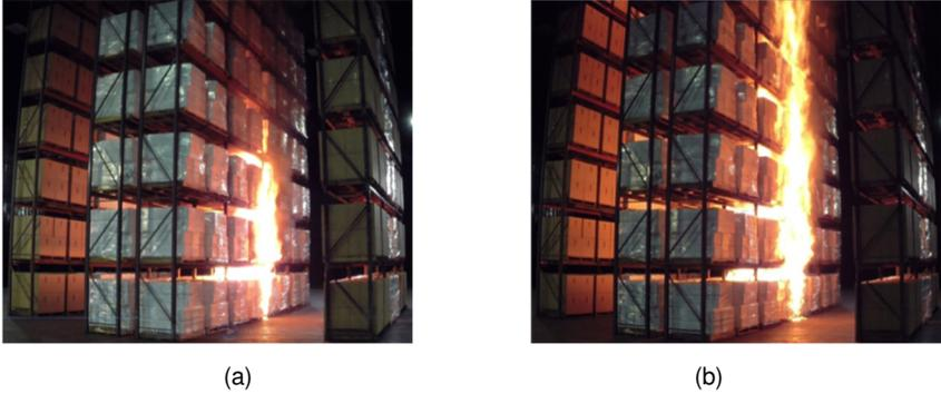
Fig. 3. (a) Fire size at electronic sprinkler activation (b) Estimated fire size at typical 101°C (214°F) ESFR sprinkler activation.
