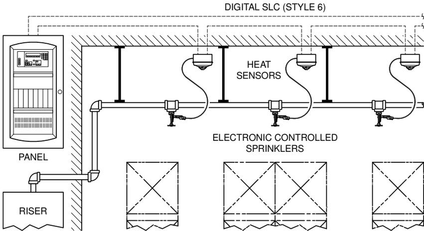
Fig. 2. Electronic sprinkler system overview as tested.
