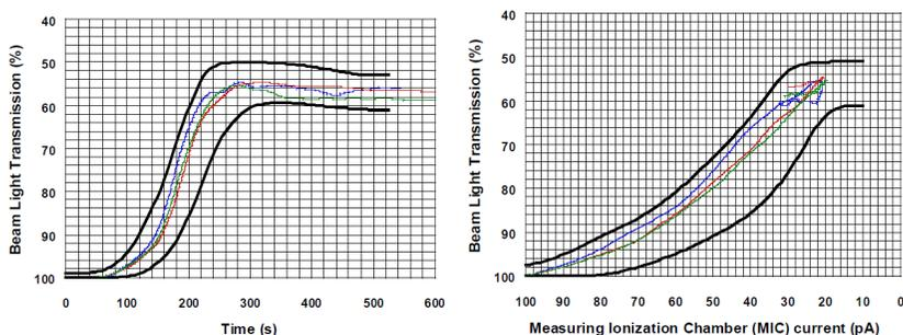
Fig. 2. Beam light transmission vs. time or MIC for flaming foam experiments.
