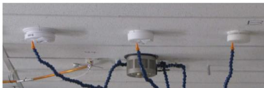
Fig. 1. MIC and smoke alarms mounted on the ceiling.
