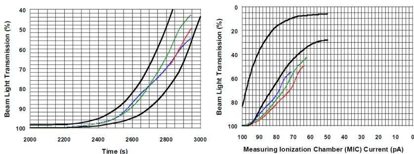
Fig. 3. Beam light transmission vs. time or MIC for smoldering foam experiments.
