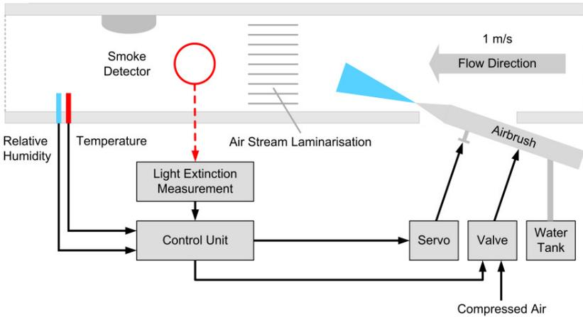
Fig. 5. Duct type test apparatus for water fog tests.
