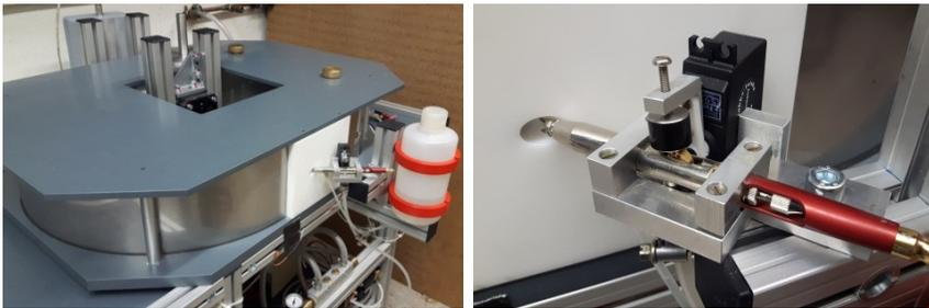
Fig. 4. Duct type test apparatus for water fog tests.
