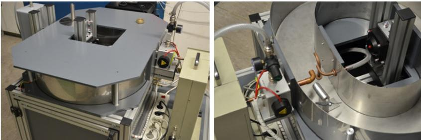
Fig. 1. Duct type test apparatus for dust tests.
