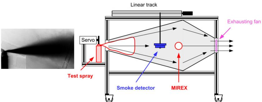
Fig. 7. Test apparatus for spray tests.
