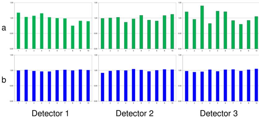
Fig. 6. RTV (Response Threshold Value)  $m$  [dB/m] of detector 1 - 3 normalized to the mean value of 10 measurements.
