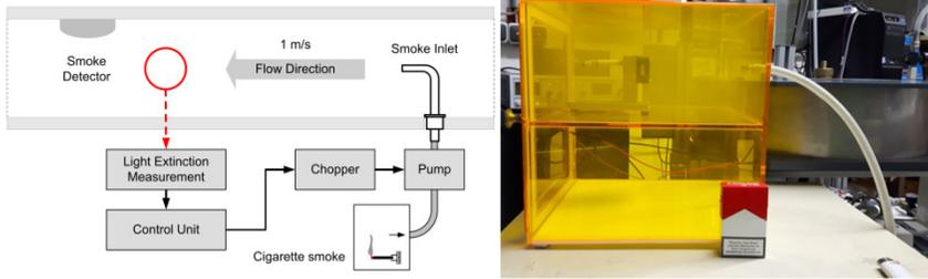
Fig. 3. Test equipment for cigarette tests.
