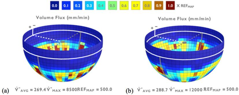
Fig. 1. Measured volume flux for two candidate deflector designs.
