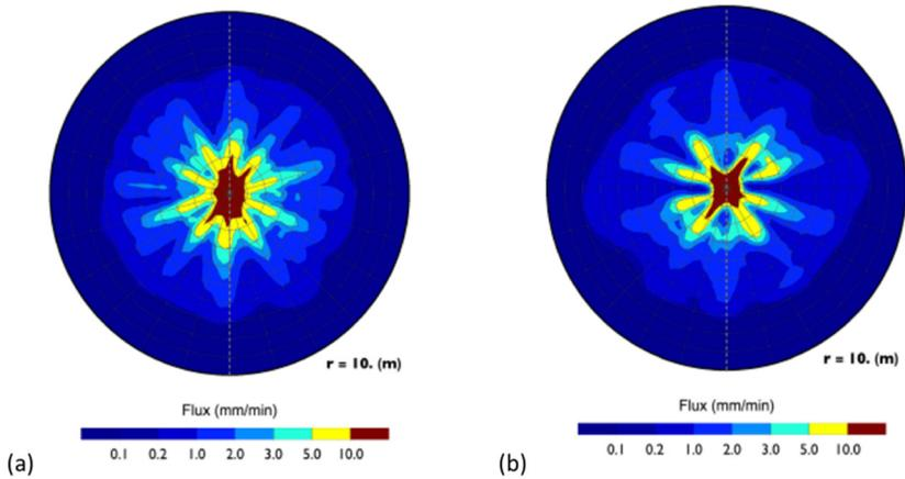
Fig. 3. Dispersion simulations for candidate sprinklers at 9.1 m (30 ft)
