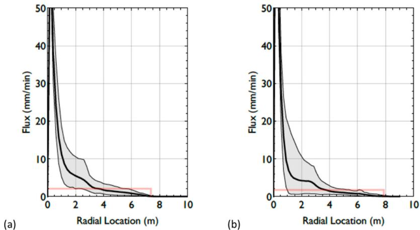
Fig. 4. Average radial flux profile with maximum and minimum flux limits.
