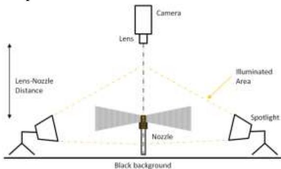
**Figure 5 Test setup optical measurements**
