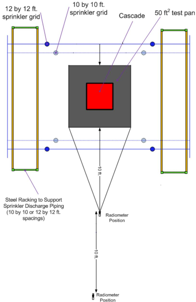
**Figure 2 – Test layout plan view.**
