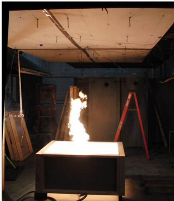
Figure 3-12 – Shroud and reduced plume lean for Test 6
