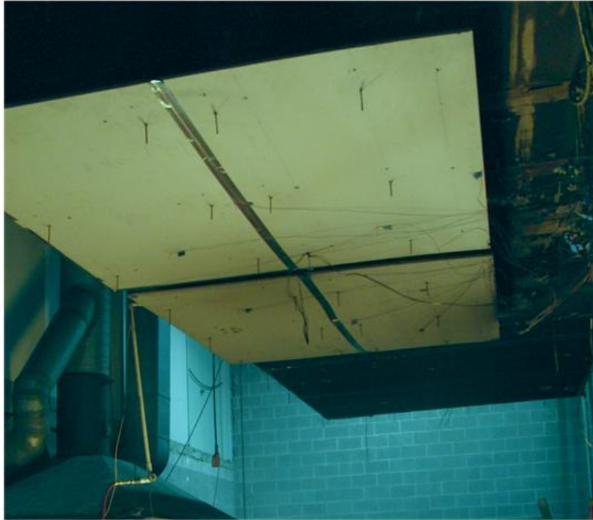
Figure 3-2 – Clouds mounted on moveable ceiling
