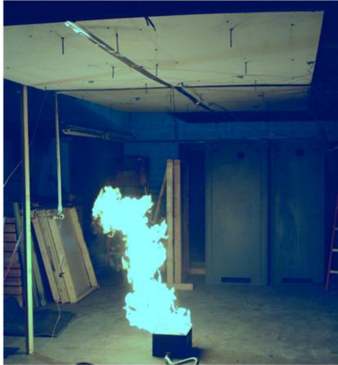
Figure 3-11 – Plume lean during first attempt at Test 6
