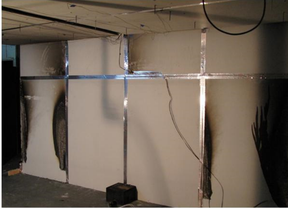
Figure 3-3 – Setup for test 3 showing the two free standing walls
