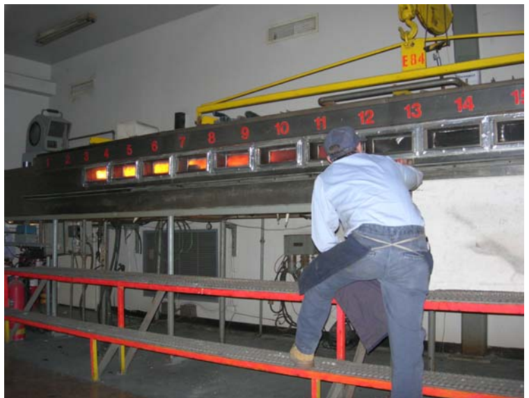
Photo 1 - Steiner Tunnel Test Apparatus
