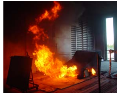
Figure 2. Pool fire underneath
